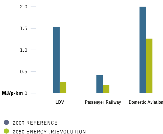
figure 11.3: world average (stock-weighted) passenger transport energy intensity for 2009 and 2050
