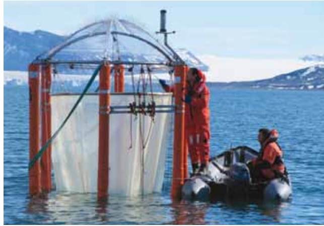
EPOCA project staff working on a mesocosm enclosure during a CO 2 perturbation experiment in the high Arctic off Svalbard.
