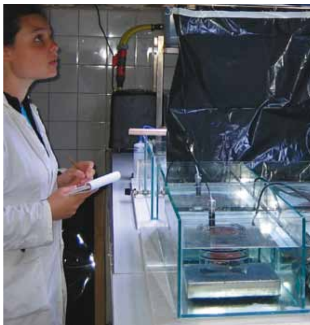
Experiment investigating the effect of ocean acidification and elevated temperatures on coralline algae.
