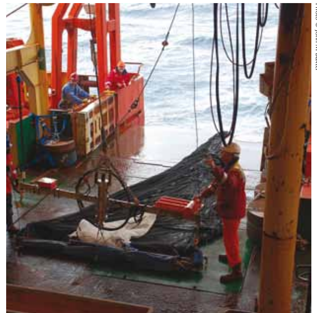
Retrieving a midwater box trawl sampling for pteropods in the Antarctic.
